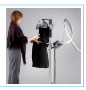
Side stand for touch up and folding. This stand makes operations faster and easier by avoiding transfer to a different touch up station. The L564 includes a handy all-steam iron, and it plugs directly into Pantastar, with no need for new electrical lines or plumbing. After touching up the trousers, the operator transfers them easily to the hanger. The L564 does not require special hangers.
